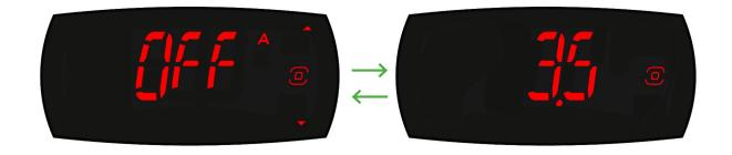
2 When the appliance is **OFF** the screen display will alternate between OFF and the current AIR/LOAD temperature, as above.
