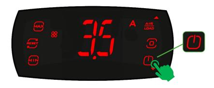
After unlocking the controller, press the **POWER** icon to turn **OFF** the appliance.
