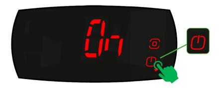
If the appliance is switched off, unlock the controller and press the POWER icon to turn ON - The screen display will show ON.
