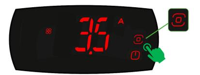
1 Press and hold the navigation button for 3 seconds
